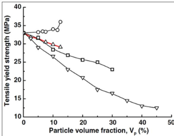
Fig. 5 – Dimensional effect of the spheric particle on the Yield strength of the PP-CaCO<sub>3</sub> composites. Particles Diameter : (○) 10 nm, (Δ) 80 nm, (◻) 1.3 μm e (▽) 58 μm.
