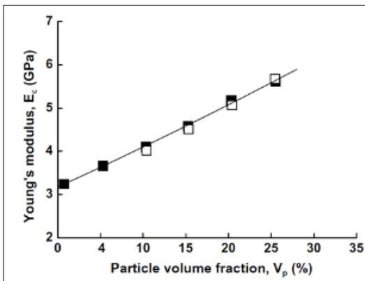
Fig. 3 – PS with Glass particle composite with excellent (□) and poor (■) surface adhesion
