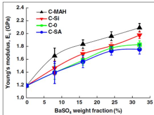
Fig. 4 – PP-BaSO<sub>4</sub> composite with different surface treatment: BaSO<sub>4</sub> without treatment (C-0); BaSO<sub>4</sub> treated with 1% stearic (C-SA); BaSO<sub>4</sub> treated with 1% silan AMPTES (C-Si).
