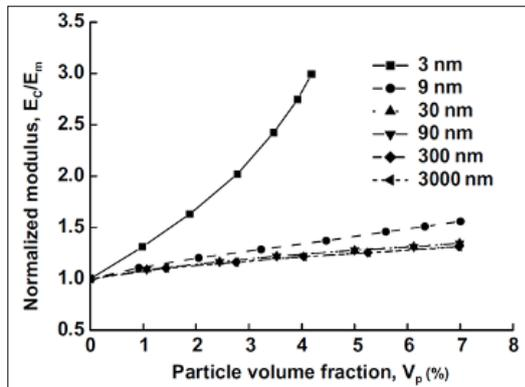
Fig. 2 – Elastic Modulus in dependence of the Volume Fraction
