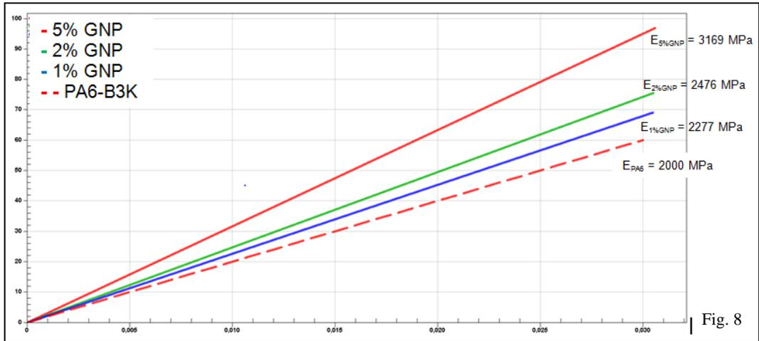
It must be highlighted that the introduction in the matrix of the 1% of the GNP gives an improvement of about 13 % of the stiffness of the matrix PA6-B3K. In Figure 9 you can see the different density of GNP for each Vf.
